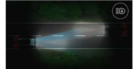
automatic main/dipped beam headlight activation. This system works using a camera that analyses light flows based on lighting and traffic conditions.
