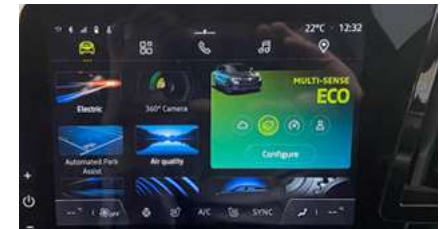
eco mode. This function makes the car as environmentally efficient as possible. It acts upon certain power consuming systems in the vehicle (heating, air conditioning, power-assisted steering etc.) and on certain driving actions (acceleration & gear changing).
